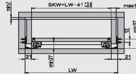
Installation for drawer with max 19mm thick drawer side
